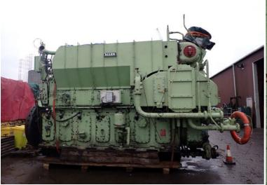
PORT MAIN ENGINE NO.4 FROM AFT LGE END SHELLS 4.5MM O/SIZE
