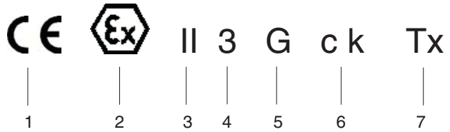
Fig. 15 Explosion protection labeling on the pump (equipment group II, category 3)
